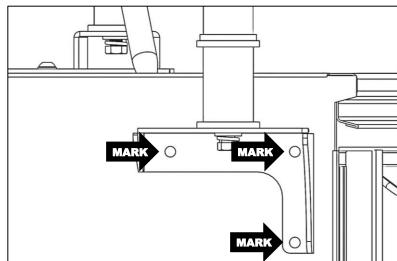
• Using three 3/8" x 1" button head screws, three 3/8" washers, and three 3/8" lock nuts for each side, securely fasten rear feet to rear of service body.
