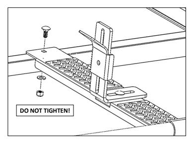
• Drill through round tube using a 7/32" drill bit.
