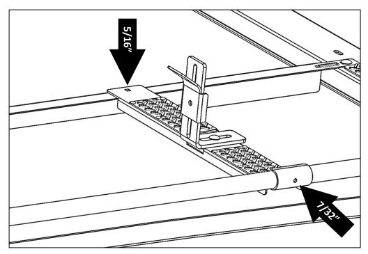
LOOSELY bolt stepladder bracket to the cross support angle bracket using one 5/16" x 3/4" carriage bolt, 5/16" flat washer, and 5/16" lock nut.
