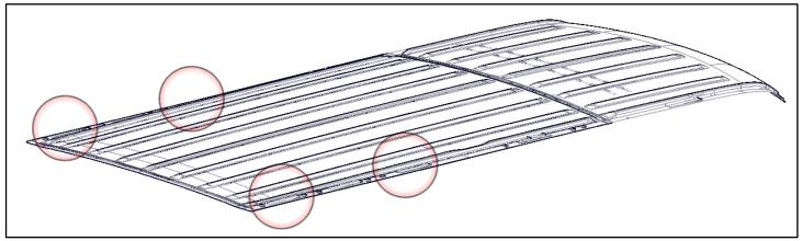
• Slide U-nut over the mounts in the locations shown. In the forward most of the two locations, only install one U-nut.
