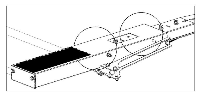
• Typically, the ladder hook on the front bow is installed on the threaded stud closest to the end of the bow.
