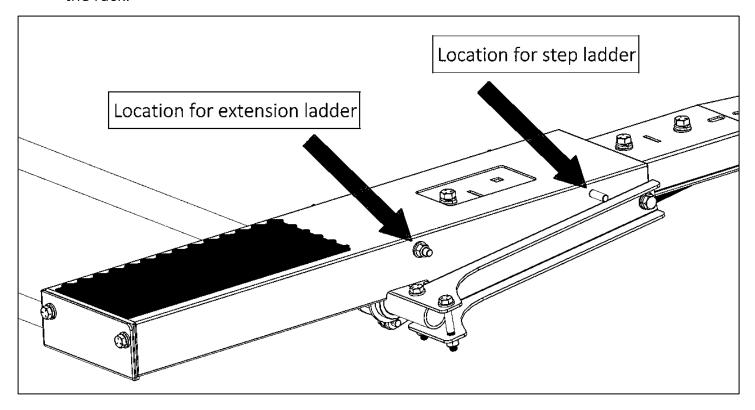
• When using an extension ladder, place the ladder hook at the threaded location closest to the end of the pan.
