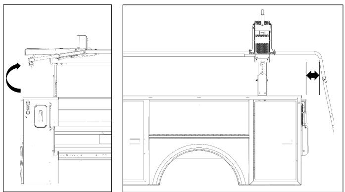
• Ensure clearance below each upright foot location, inside service body cavity, for mounting plate to be installed below each upright foot.
