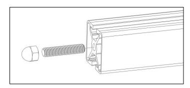
Screw the other extrusion onto the other end of threaded stud.
