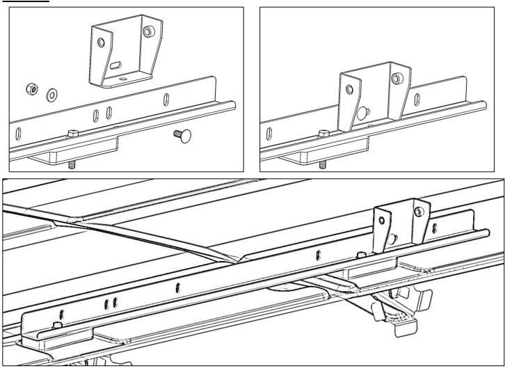
Notice the short feet are installed at the front.
