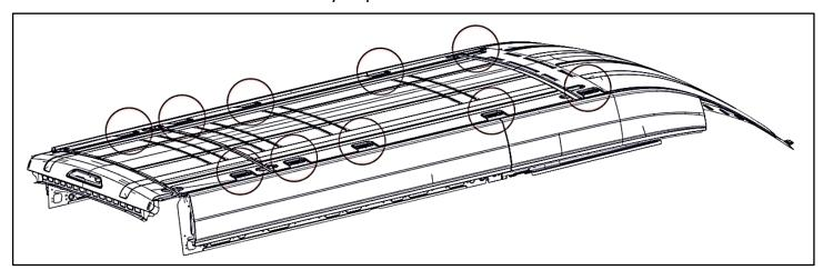
\*\* We recommened using the rear most, middle and front most mount location on the Transit installations shown below. \*\*
