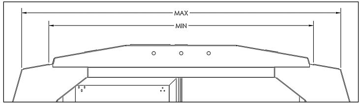
• Determine the best mounting width. Locate the corresponding slots on the ladder rack bow. Be sure the same slot is used at both ends of the ladder rack bow.
