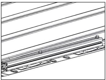
• Bolt long section of rail at the front of the van. Bolt through the rear two holes using M8 x 55mm HH (1), M8 split lock washer (2), M8 flat washer (3) and into the M8 U-Nut (4). The hole closest to the cut goes towards the rear. Put Anti-Seeze on all threads.
