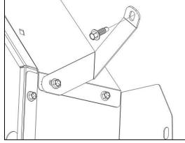
In the remaining locations along the wings, as shown, secure wings to the "B" pillars using 5/16" x 1" self-tapping screws.
