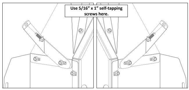
• Use **5/16" x 1"** self tapping screws, secure the remaining three locations along the wings to each "B" Pillar.
