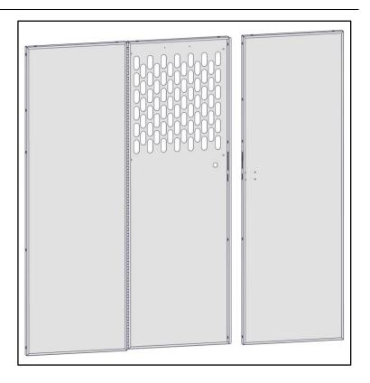
• Bolt together using a 1/4"-20 x 5/8" hex head bolts and 1/4" nyloc nuts. Place two 1/4" flat washers in between the two parts.
